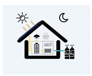
▲ Winter: Stored hydrogen powers electricity and heat via the fuel cell
